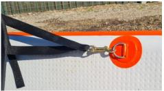
Using the brass clips, clip them to the silver D rings on the kayak. Adjust the straps till tight, and the back rest supports well.
