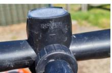
Make sure the release valve toggle on the kayak valve is popped out in the closed position.
