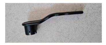
YOU MUST USE your thumb to hold the head of the tool firmly down, while you use your other hand to turn the tool, if the tool becomes loose while turning the teeth can break.
